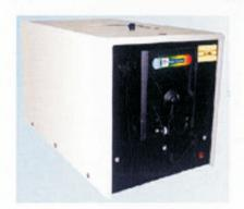
Spectro - Photometer for Strength & Shade Testing
